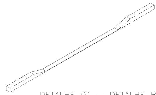
DETALHE 01 – DETALHE REBAIXO ENTRADA DE GARAGENS S/ESCALA
